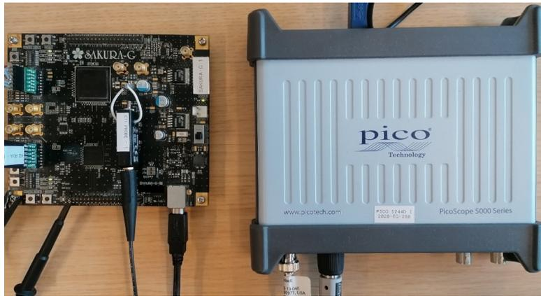
**Figure 3:** Dynamic power setup including a Sakura-G board and a PicoScope 5224D.
