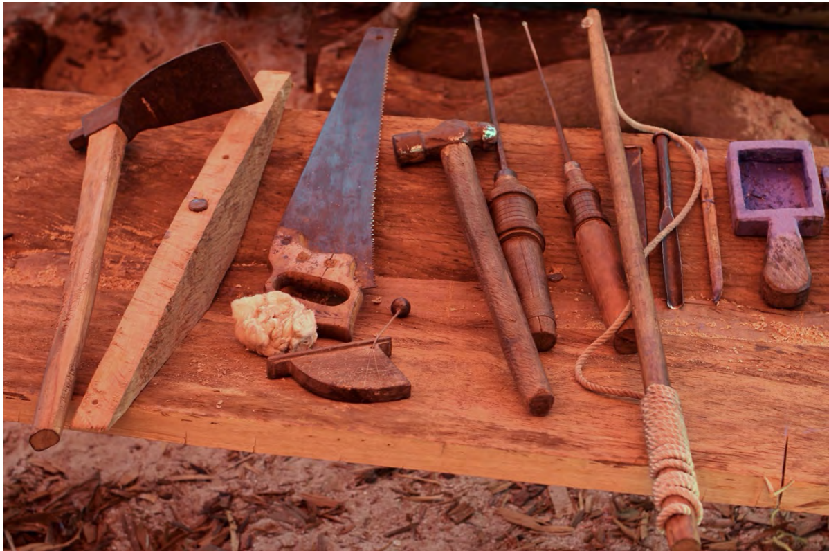
Figure 3. A boat builder's set of basic tools, Zanzibar. Photograph by T. Marchand.
