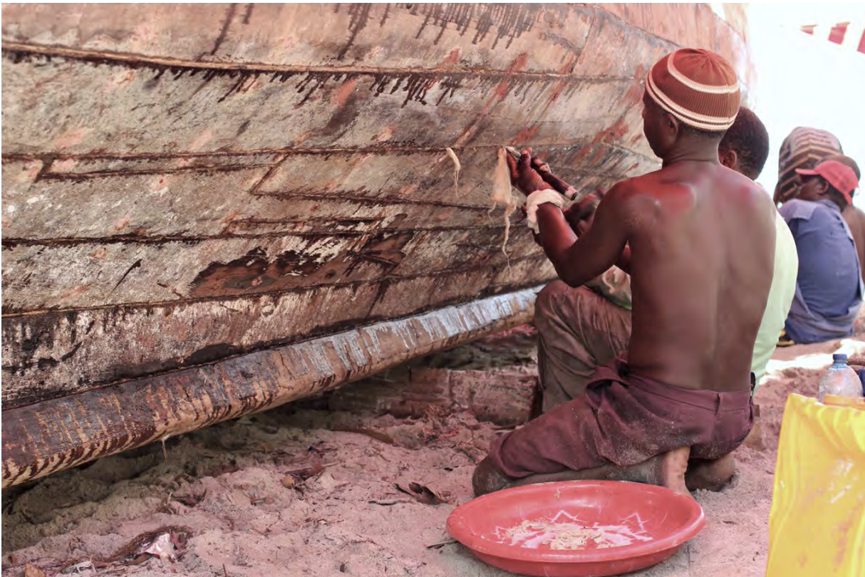
Figure 5: Boat builders using caulking irons and wooden mallets to fill the seams between planks with cotton soaked in shark oil, Zanzibar. Photograph by T. Marchand.
