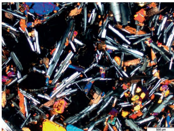
Figure 16. Dominant structure is prismatic laths of anorthite in KT20471.
