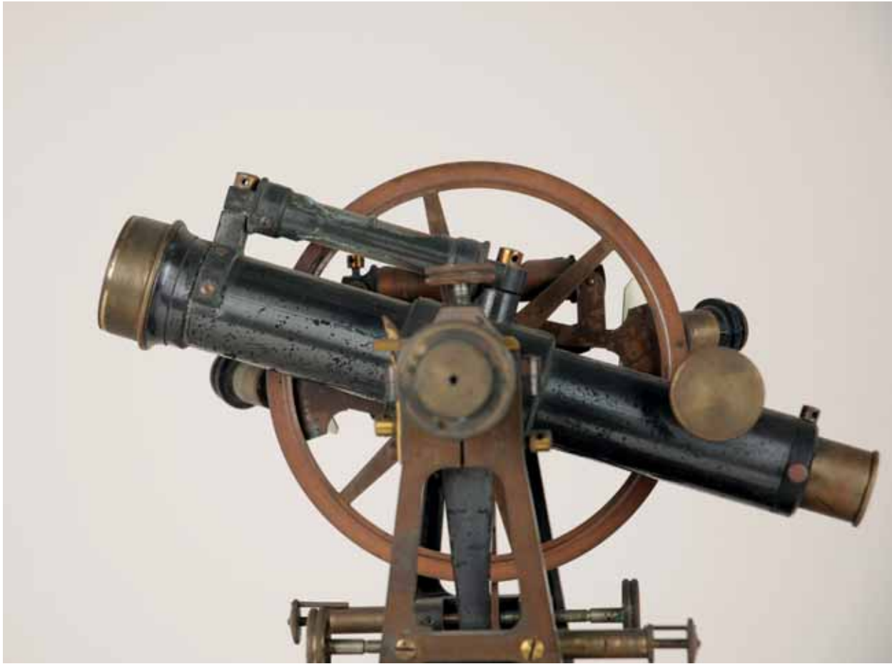
Figure 5. Repetition theodolite DBM Inv. no. 030150289000. Photo: M. Braun.
