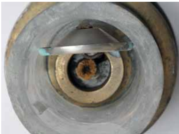
Figure 2. View from top into the opened lamp (Figure 1): corrosion of the reflector at contact zones to glass. Photo: A. Schorpp.
