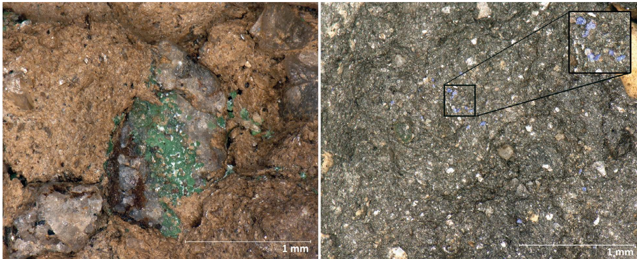
Figure 21. In some ceramic fragments from Göttschen-Brixen im Thale, secondary minerals of fahlore were found embedded in the ceramic matrix (temper material). Left: malachite (green), right: azurite (blue). Photomicrographs taken by U. Töchterle and R. Lamprecht using Keyence VHX-6000.
