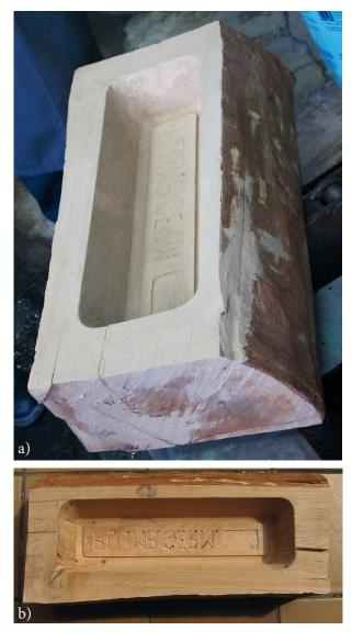
Figures 17. Wooden mould for the casting of a cuboid ingot (main type C) with a large cartouche inscription PLUMB. GERM. Photos: N. Hanel and R. Köhne.
