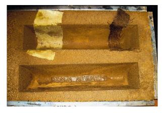
Figure 15. Clay mould for double ingot casting. Scraps of tissue inserted into the upper ingot. Photo: R. Köhne.
