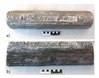
Figure 13. a. Top of the modern lead ingot with cartouche inscription. Traces of the cracked and repaired mould in the right half of the photograph; b. Front of the lead ingot with horizontal casting lines. Photos: N. Hanel.
