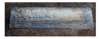
Figure 16. Modern lead ingot with an impression of the tissue remains (top left) and casting lines. Photo: R. Köhne.
