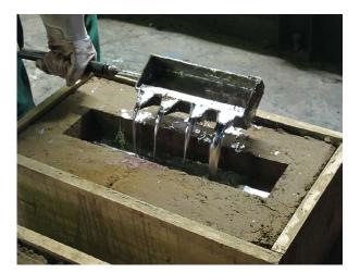
Figure 8. Pouring the liquid lead into the clay mould, using a metal four-pronged casting ladle. Photo: N. Hanel.
