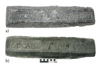
Figure 21. Two Roman lead ingots from Wade Street, Bristol, with identical casting defects in the centre of the cartouche. Photos: CRLI.
