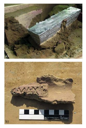
Figure 14. a. Removal of the cooled lead ingot from the clay mould; b. Rest of the cartouche inscription after the ingot casting. Photos: N. Hanel.
