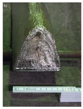
Figure 20. Modern lead ingots from the ceramic casting mould (a) with interrupted fillings, b. in the course of one casting process. Photos: N. Hanel.
