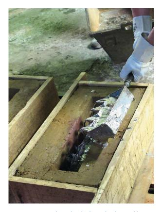
Figure 11. Pouring the molten lead into the clay mould, using a four-pronged casting ladle. In the background there is the metal vessel for removing the lead. Photo: N. Hanel.
