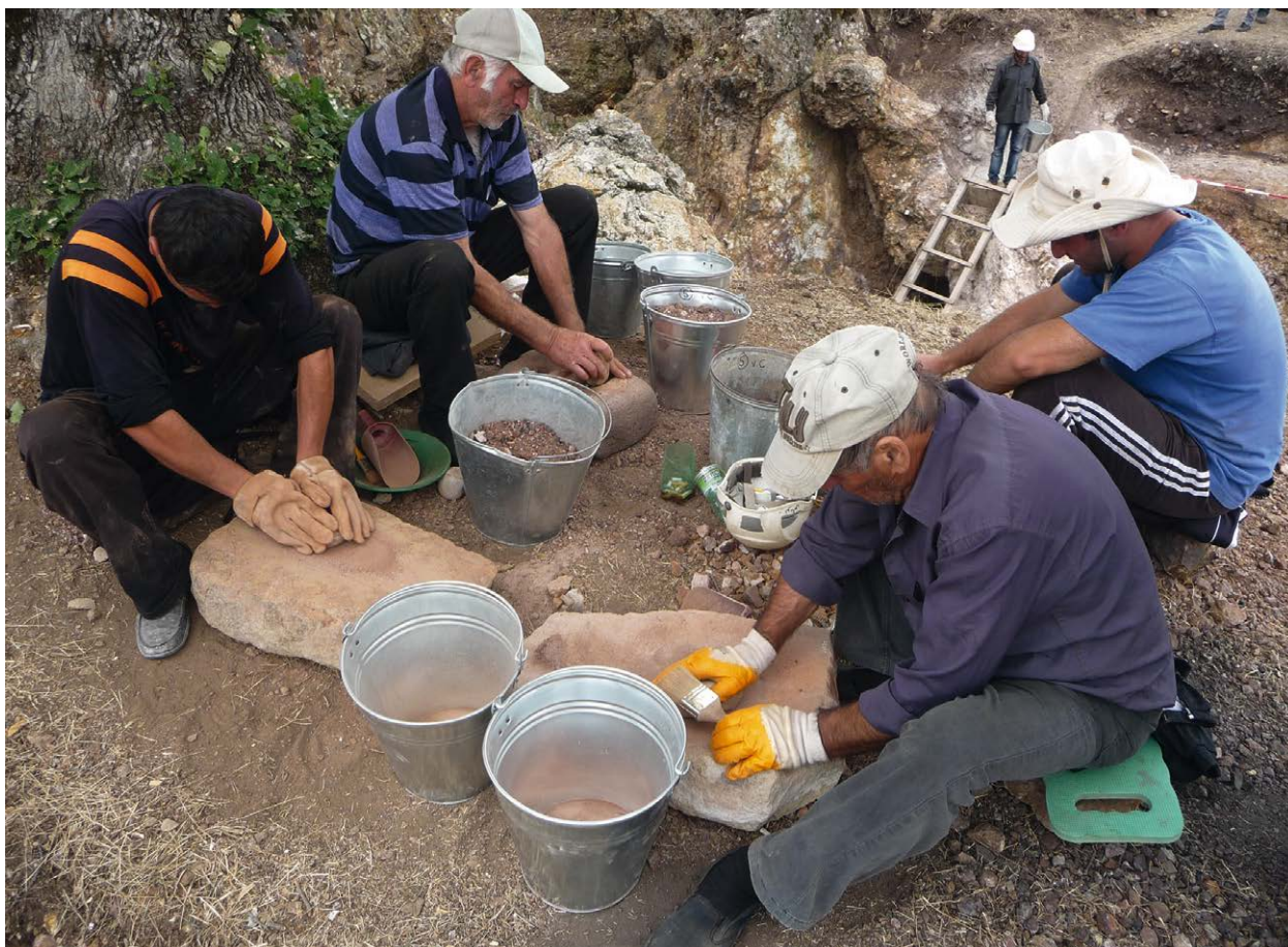
Figure 27. Grinding quartz-hematite to powder prior to gold washing at Sakdrisi in 2013. Photo: S. Timberlake.
