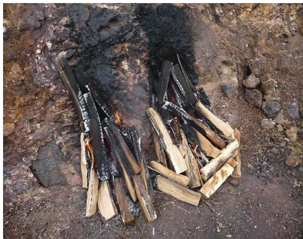
Figure 25. Firesetting on two parallel vein workings at Sakdrisi, Georgia in 2013 note the temperature probe for the firings can be seen against the rock face on the RH side. Photo: S. Timberlake.
