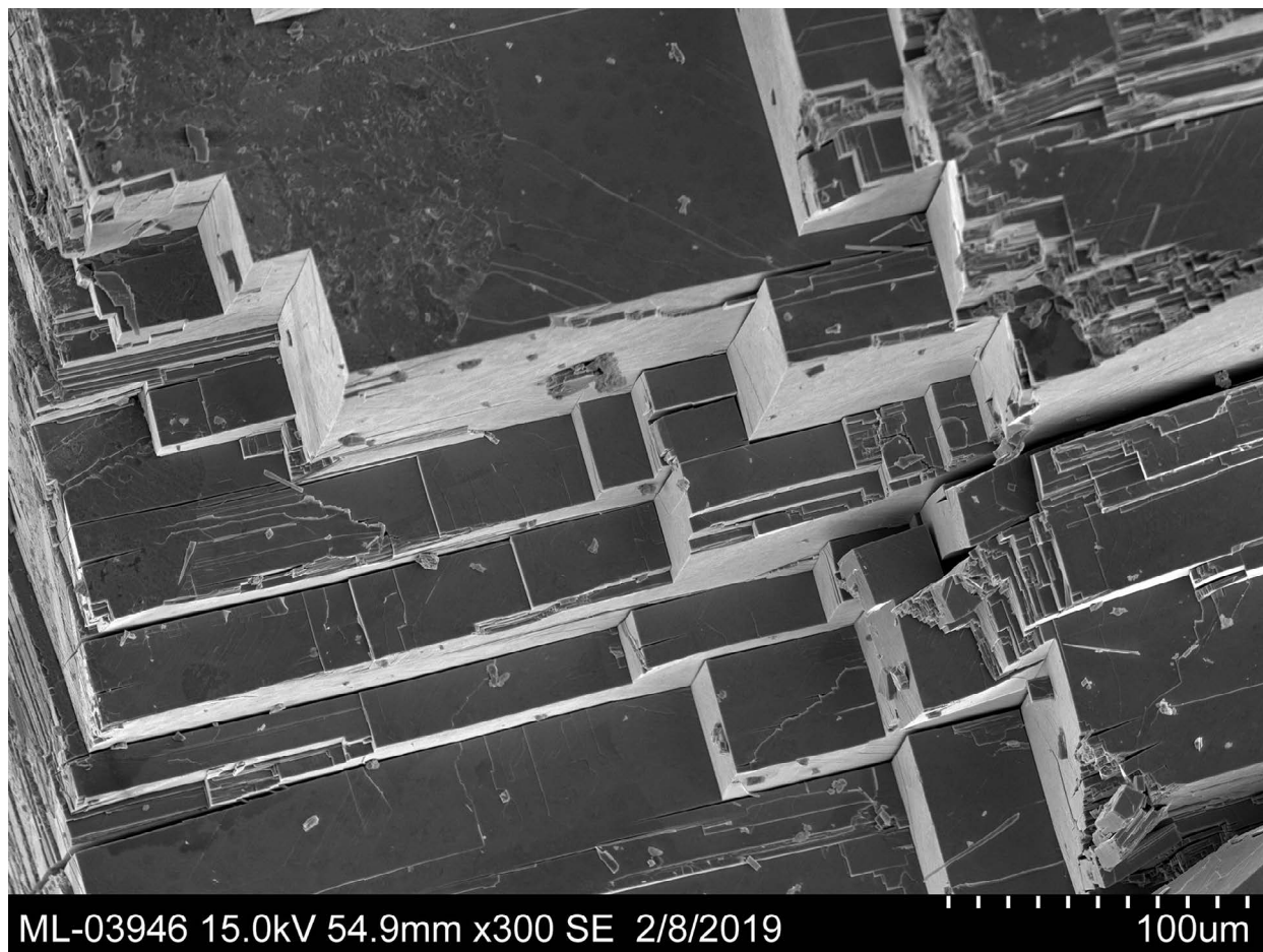
Figure 1. Fracture structure of a galena sample from Can Sadurní (13CS-H10-IIJ-11a4-92) under the scanning electron microscope (SEM). Photo: O. García-Vuelta, Instituto de Historia-CSIC, Madrid.
