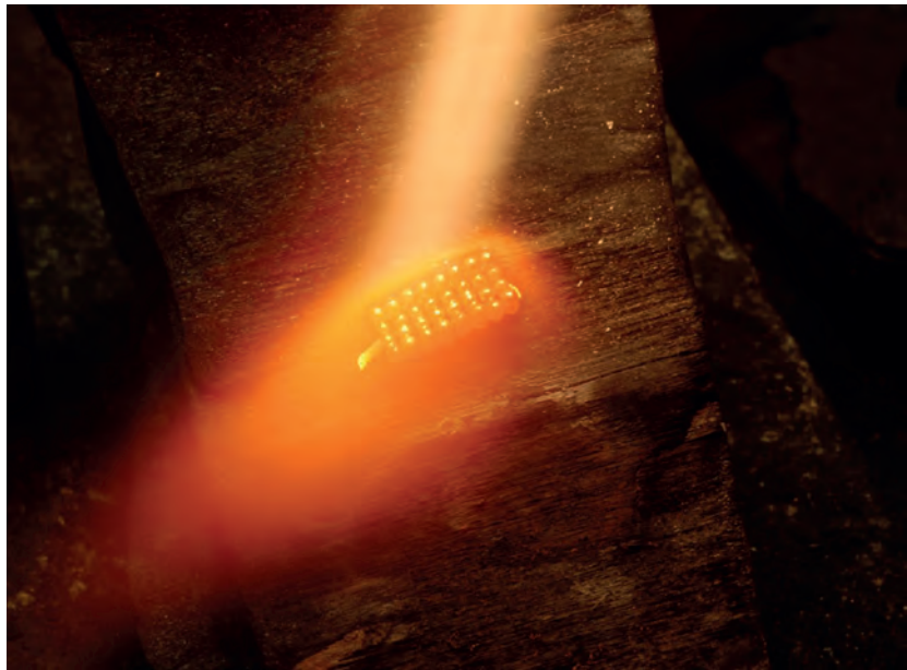
Figure 6: The final brazing, which joins the planes together. Photo: D. Loepp.
