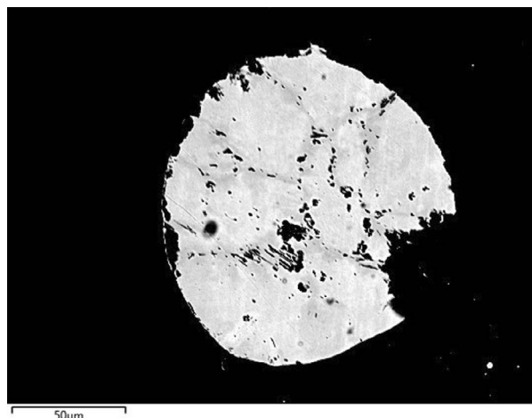
Figure 11. High contrast SEM-BSE image of FAG Prill #2 from Ind-Chn'19-Cru001D, characterized by low silicon (0.8 wt.%) and phosphorus (0.1 wt.%) concentrations. The prill has a cementite-pearlite microstructure with inter-granular porosities and beginning corrosion. Scale: 50 µm or 500 x. Photo: M. Desai and Th. Rehren, Archaeological Science Laboratories, The Cyprus Institute.
