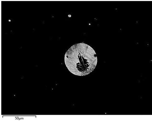
Figure 18. High contrast image of prill #8 (crucible slag film) from Ind-Ksm'19-Cru009A. Area analysis shows that the composition is low in phosphorus (0.3 wt.%). The prills shows cementite needles in austenite / pearlite matrix, indicating a high carbon content. Scale: 50 \mu\text{m} or 500 x. Photo: M. Desai and Th. Rehren, Archaeological Science Laboratories, The Cyprus Institute.
