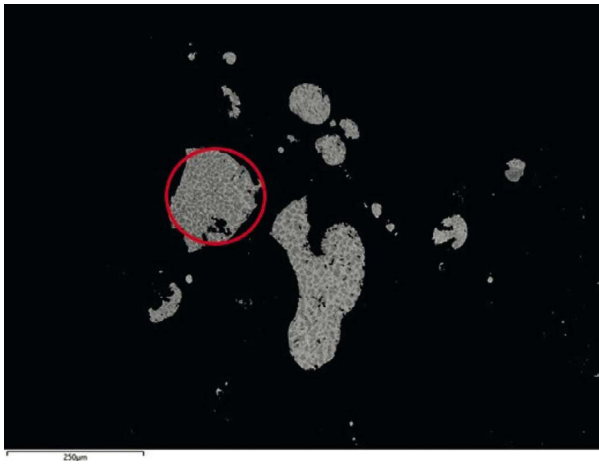
Figure 8. High contrast SEM-BSE image of prill #6 from Ind-Gur'19-Cru001B. Area analysis quantifies high silicon (~15 wt.%) and low phosphorus (~3.8 wt.%). The melt forms within temper porosity; both porosity and ceramic matrix are black due to the high contrast setting. The entire cluster of iron melts/prills shows high values of silicon (9-16.6 wt.%) and phosphorus (1.8-8.7 wt.%). Scale: 250 µm or 100 x. Photo: M. Desai and Th. Rehren, Archaeological Science Laboratories, The Cyprus Institute.
